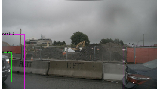
Fig. 5. Example of a model prediction error in the nuScenes autonomous vehicle dataset. This error was found via a consistency assertion between different sensor views of the same data (3D point cloud and camera data). Taken from Kang et al. [32].
