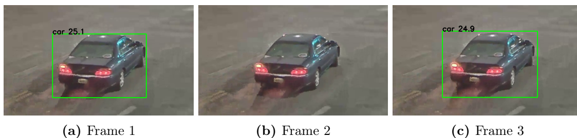
Figure 1.2: An object detection model erroneously missing the prediction of the car in the second frame. Even widely used models (SSD) fail simple checks, such as temporal consistency.
