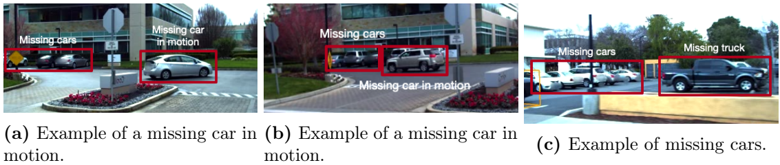
Figure 5.12: Examples of labeling errors in the Lyft dataset. The missing objects in these examples can be within 20 meters the autonomous vehicle and several are in motion: vehicles in motion are the most important to detect.
